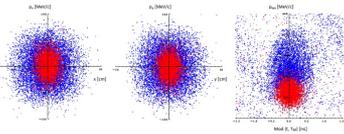
Initial 6D Cooling:  $\epsilon_{6D} \approx 60 \text{ cm}^3$  a  $\sim 50 \text{ mm}^3$ ; Trans = 67%
